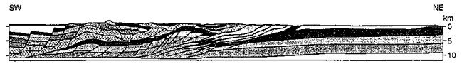
FIG. 6 - A SW to NE section of the Apennines, starting south of Naples. Several nappes are thrust against the foreland in the NE, but the whole has been eroded and affected by normal faults which creates the present topography. The three shaded layers on the foreland (right) are Cretaceous, Jurassic, Triassic. The same sequence is repeated in the upper nappe in the SE. The cross-stippled layer beneath it is another nappe with rocks of the same age (simplified after a section in Cassano & alii , 1986).
