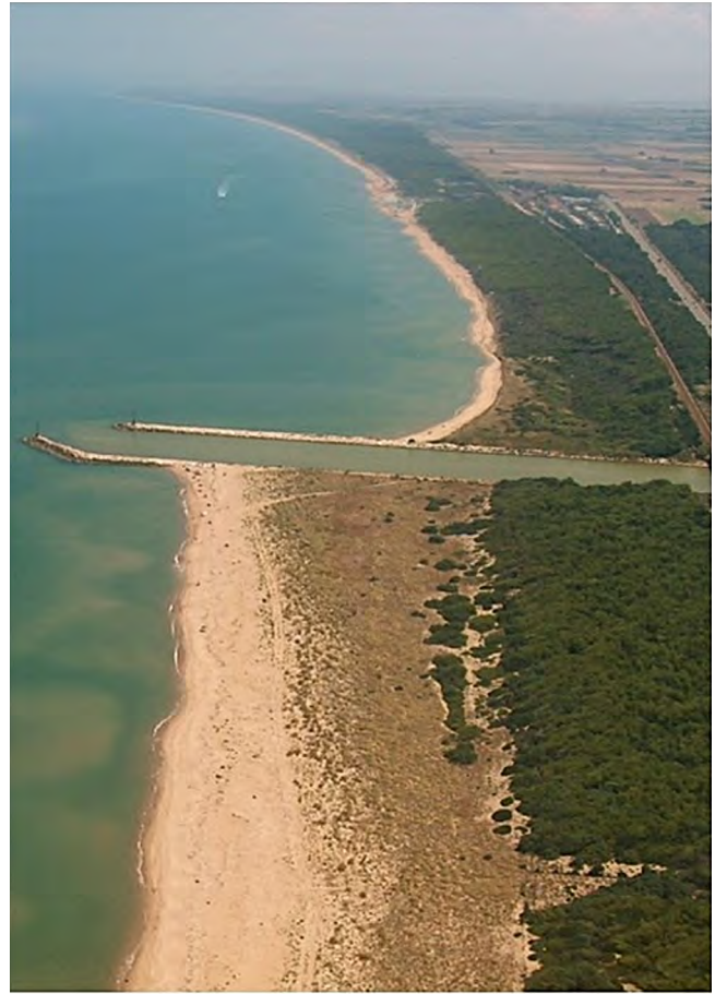
Figure 10 - Effect of the construction of a reinforced mouth on the Saccione River on the border between Puglia (Southward, on the background) and Molise (Northward, on the foreground); this results in a strong regression of the shoreline in Puglia and its disproportionate progradation in Molise in the sopraflutto area compared to the coastal drifting here directed from NNW to SSE (Photo: M.A. Caldara).
