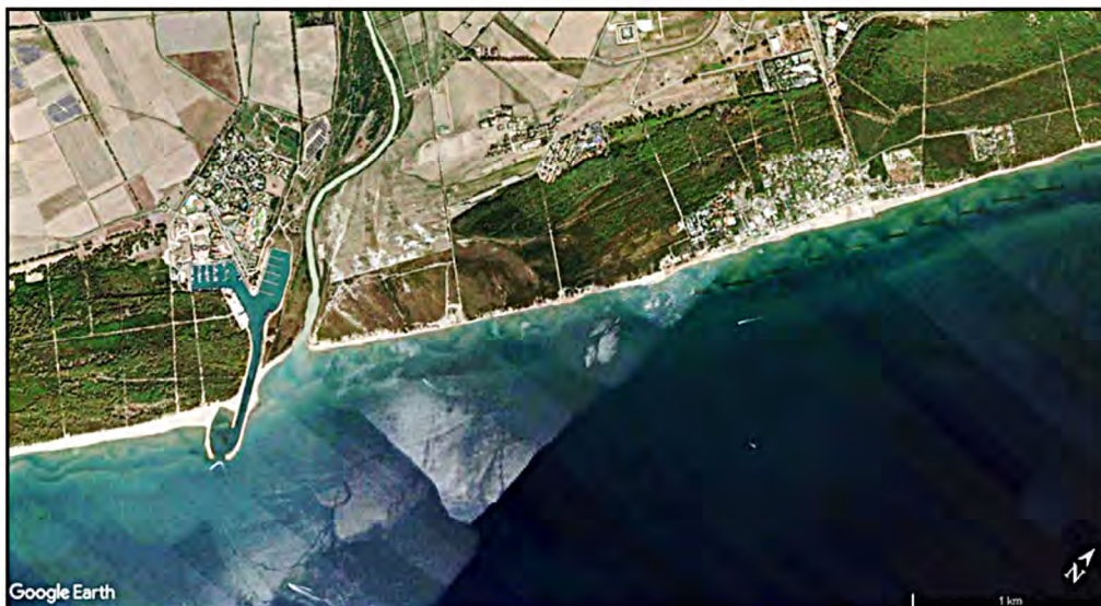
Figure 11 - 2016, July: state of the mobile coastal system at the Argonauti tourist village and harbor, built starting on the first year of XXI century, at the mouth of the Basento River (Matera, Basilicata); the progradation in the sopraflutto zone with respect to the coastal drift, here directed from SSW to NNE) and the dramatic retreat in the sottoflutto zone are evident (from Google Earth).
