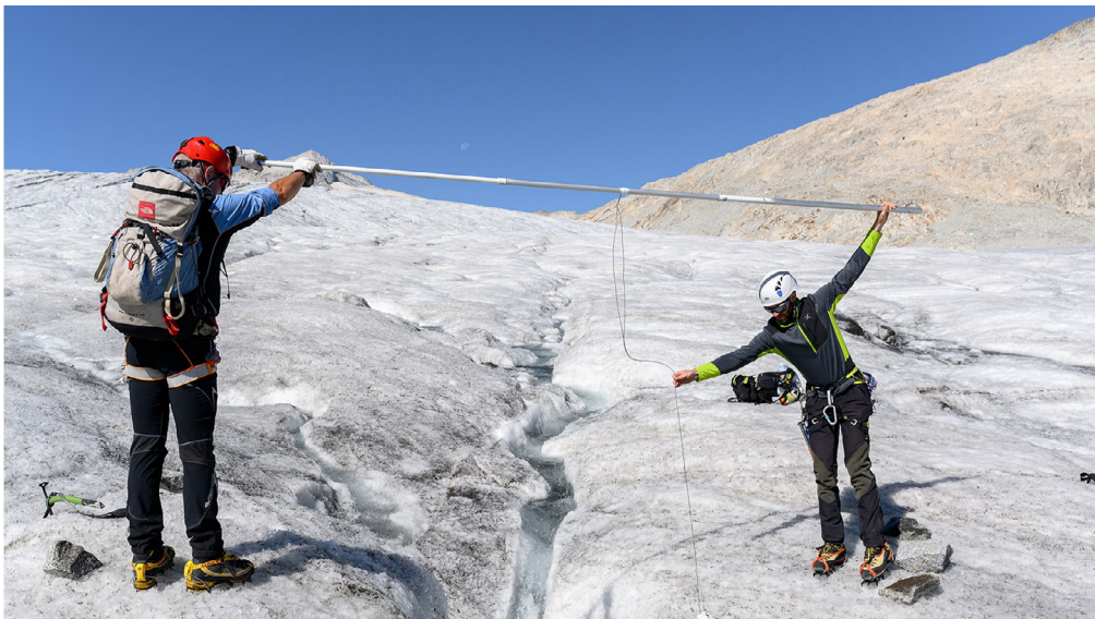
Figure 3 - Installation of the sound recorder in one crevasse of the Adamello Glacier during the 2022 campaign.
