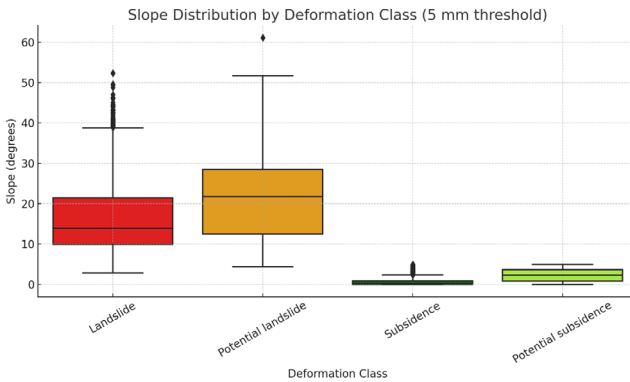
Figure 10 - Slope distribution across MAC classes using the more sensitive \pm 5 mm/year threshold. The wider spread of slope values for Potential landslides reflects the inclusion of incipient or low-magnitude movements.
