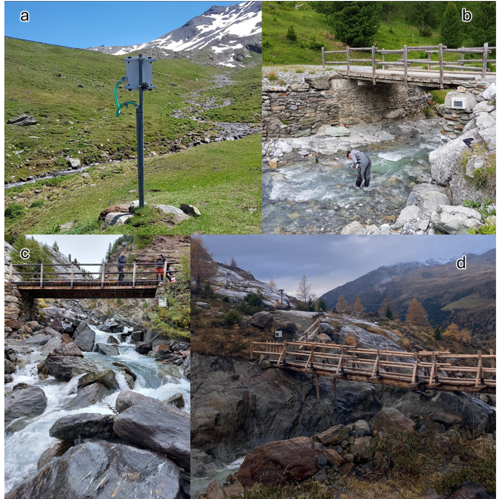
Figure 3 - Four representative stations of IdroStelvio network: a) the highest altitude station, Braulio Stelvio, monitoring the smallest stream, ca. 1 m wide, b) Zebrù station, located in a low slope area, allowing safe measurements of geometry and discharge, c) Forni Cedec station, located in a very steep area, where discharge measurements are made difficult by turbulence, d) Forni Monte station, downstream Forni glacier, where the discharge regime is strongly related to air temperature in summer.
